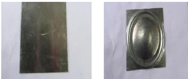
Fig 2.2: Initial specimen on which test is conducted Fig 2.3: Specimen after deformation due to applied load
